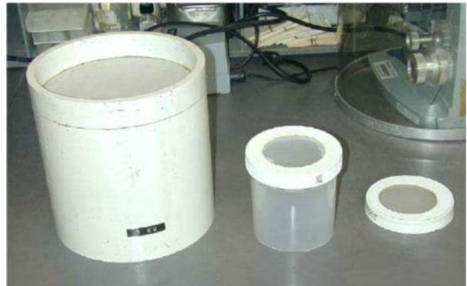
**Figure 6.** Homemade sieves
